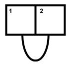
Opening the REPO connection will disable the UPS. Manual restart using the front panel is required after the REPO connection is closed again.
